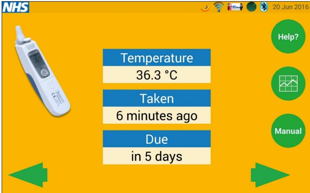
The screen shows the most recent reading, how long ago that reading was taken, and when the next reading is due.
